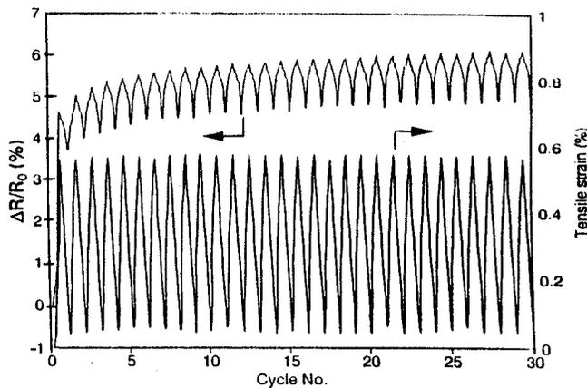
Fig. 1  $\Delta R/R_0$  vs. cycle No. and tensile strain vs. cycle No. during first cyclic tension.
