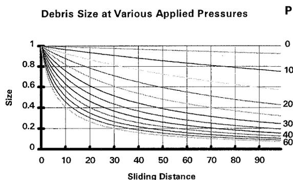
Figure 1: Plot of a series of curves showing the attrition of particle size with sliding distance for a range of pressures. Units are arbitrary.
