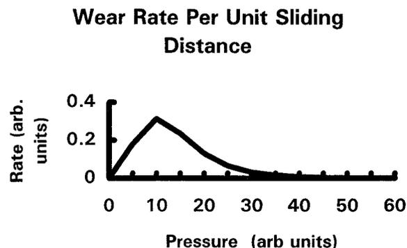
Figure 2. Wear rate per unit sliding distance vs pressure. Units are arbitrary. The plot is intended to show that a peak in wear rate is predicted from the elements of the model.
