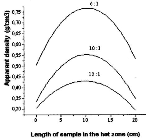
Figure 2. Apparent density as a function of length of sample The variation of apparent density along the sample length as function of different N<sub>2</sub>/CH<sub>4</sub> ratios.
