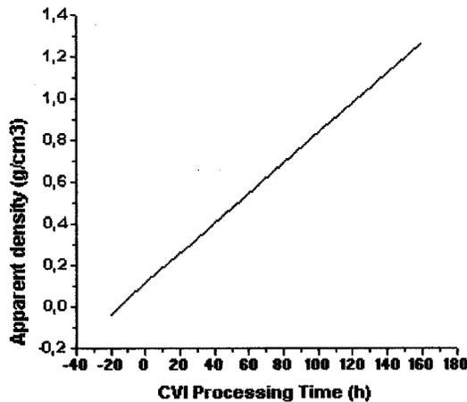
Figure 1. Apparent density as a function of CVI processing time. it increases with CVI processing time. N<sub>2</sub>/CH<sub>4</sub> volume ratio: 12:1.
