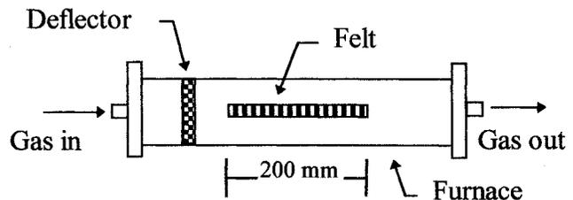
Figure 1 - Experimental set up for CVI processing.
