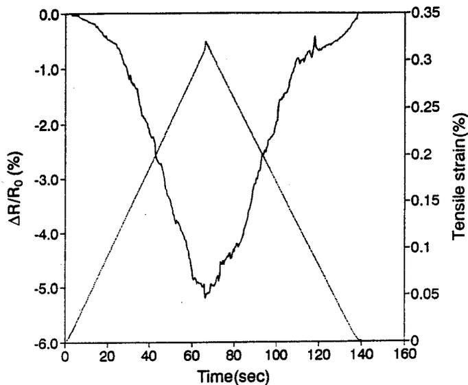
Fig. 2 Plots of  $\Delta R/R_0$  vs. time and strain vs. time during tensile loading and unloading for single carbon fiber in epoxy. Solid curve:  $\Delta R/R_0$  vs. time. Dashed curve: tensile strain vs. time.
