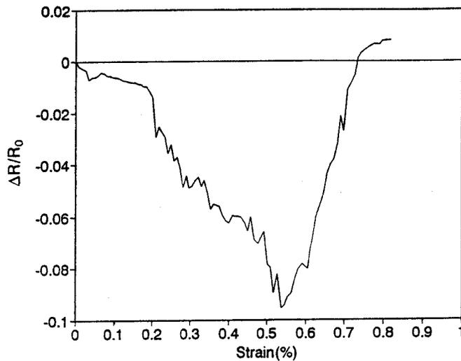
Fig. 1  $\Delta R/R_0$  of single carbon fiber in epoxy under tension.
