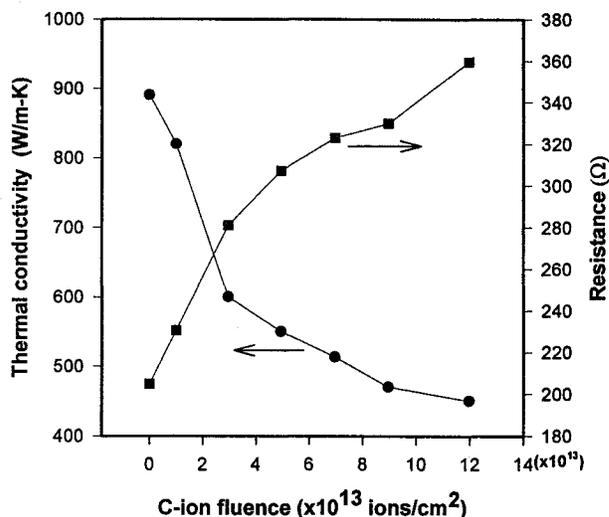
Fig. 1 The thermal conductivity (circles, left-hand axis) and the electrical resistance (squares, right-hand axis) of a single K1100 filament as a function of Carbon ion fluence.
