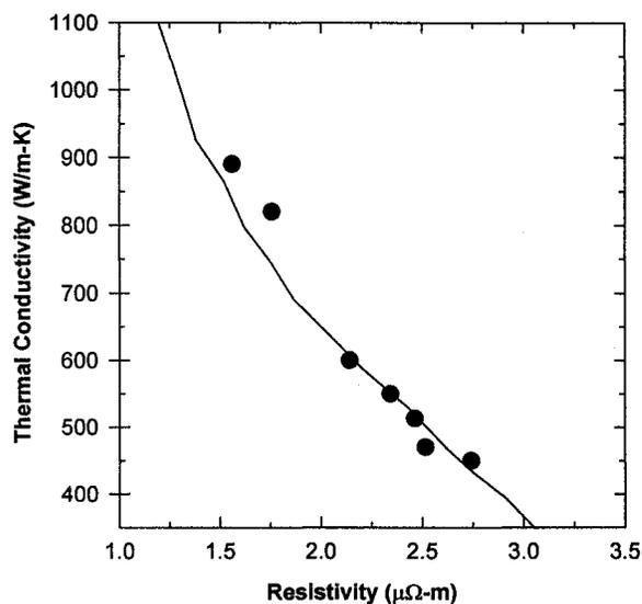
Fig. 2. The thermal conductivity vs the electrical resistivity for the implanted fiber from Fig.1 (circles). The curve is the widely used universal TC-ER relation.<sup>1</sup>
