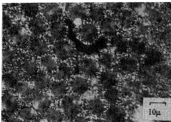
Fig.5 Polarized optical micrograph of carbon-carbon composite(HTT 2700 o C) made with PANOX fiber and coal tar pitch
