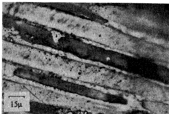
Fig.2 Polarized optical micrograph of carbon-carbon composites(longitudinal section) made with PANOX fiber and coal tar pitch(HTT 550 o C)
