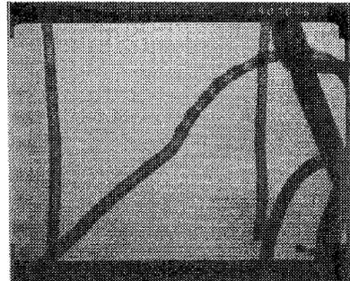
Fig. 2. Bamboo-like structure in VGCF.
