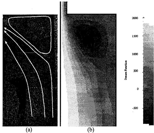
Figure 2. Comparison between an experimental picture of circular flow to one contraction flow of AR mesophase (a), and numerical calculations based on White-Metzner model (b). Note that color pictures clearly showing the flow pattern will be presented at the Conference.
