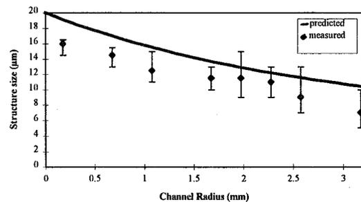
Figure 3. Comparison between predicted and measured size of the transverse texture in the upper channel.
