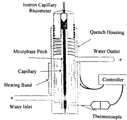
Figure 1. Design of mesophase pitch quenching apparatus.
