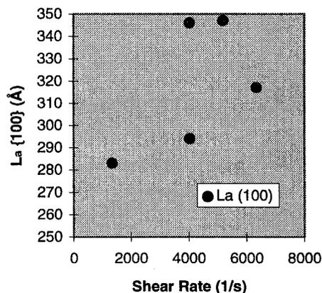
**Figure 4.** Crystal size, based on the 100 peak, as related to shear rate within a flat-entry capillary.
