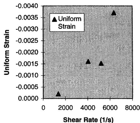
**Figure 3.** Uniform strain dependence on shear rate for fibers spun using a flat-entry spinneret.
