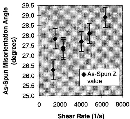
**Figure 1.** As-spun misorientation angle as a function of shear rate for fibers spun using flat-entry capillaries.
