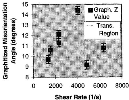
**Figure 2.** Graphitized misorientation angle vs. shear rate for ribbon-shaped AR-mesophase pitch-based carbon fibers spun using a flat-entry spinneret.
