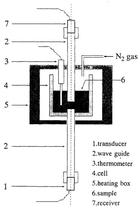
Fig. 1. Schematic diagram of a main part of the ultrasonic apparatus.
