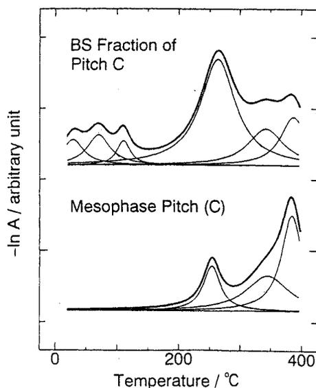
Fig. 2. The variation of  $-\ln A$  with temperature and separated peaks for mesophase pitch (C) and benzene-soluble fraction of pitch C
