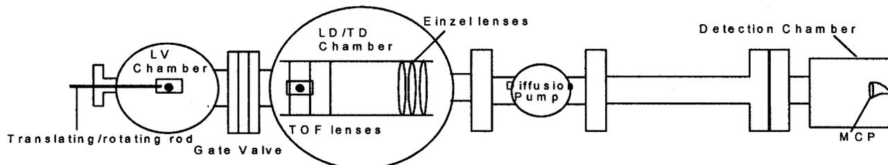
Figure 1. Diagram of our LV/LD/TD TOF-MS
