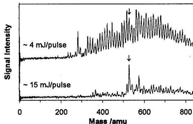
Figure 1. Photoionization mass spectra of neutral Ti/C clusters produced with two different vaporization laser powers at a constant photoionization condition. The peaks corresponding to  $Ti_8C_{12}$  are marked by arrows ( $\downarrow$ ).
