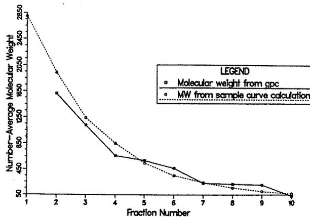
Figure 2. The molecular weight of the naphthalene pitch fraction is compared to the molecular weight extrapolated from the original sample curve.
