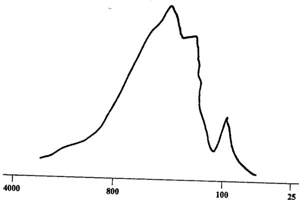
Figure 1a. GPC curve of naphthalene pitch.
