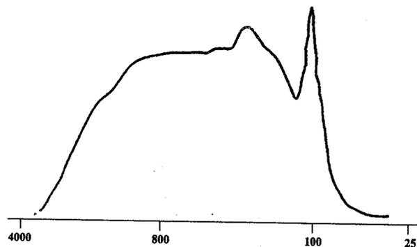
Figure 1c. GPC curve of pyrolysis tar pitch.
