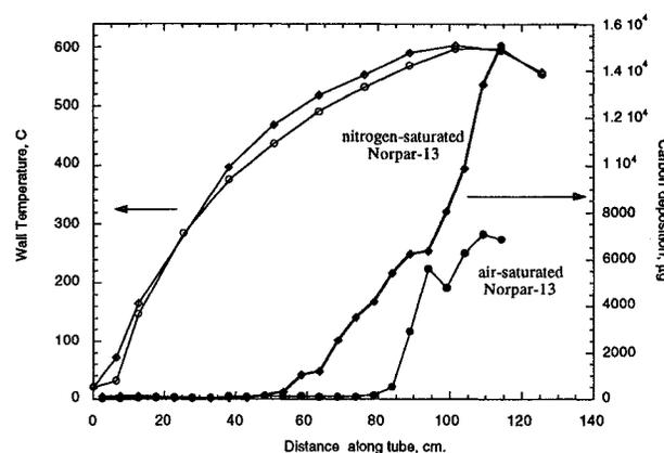
Figure 1. Temperature and carbon deposition profiles on 304 stainless steel tubes.
