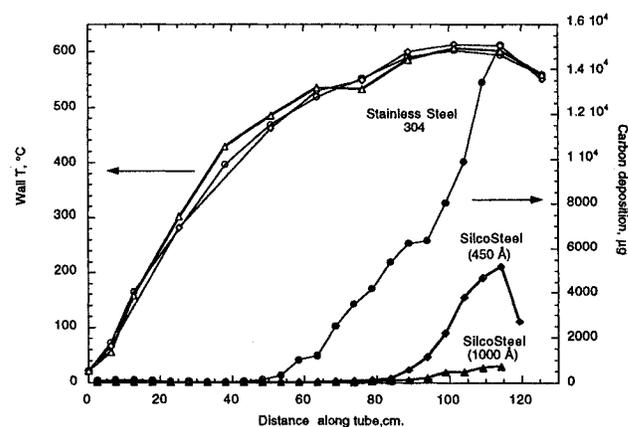
Figure 2. Temperature and carbon deposition profiles on 304 stainless steel and SilcoSteel tubes.
