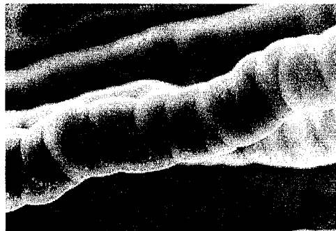
Figure 1. Different shapes of Vapour Grown Carbon Fibres. a) 'Perfect cylinder'; b) 'Quasi-perfect cylinder'; c) 'Crenulated'.
