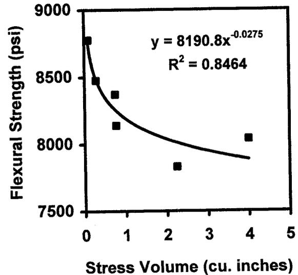
Figure 1. Dependence of flexural strength on the tensile volume for specimens of various sizes from the same material.
