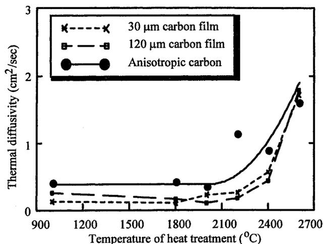
**Figure 2.** Plots of thermal diffusivities of polyimide carbon films and anisotropic carbon as a function of the temperature of heat treatment.
