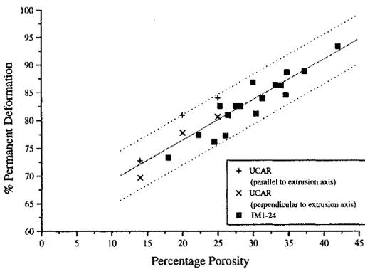
**Figure 4.** The effect of porosity on the permanent deformation of graphite, for a 1kN indentation cycle.
