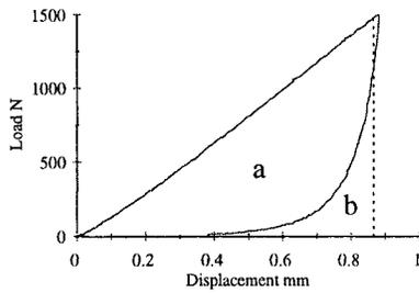
**Figure 3.** Characteristic hysteresis loop for unoxidised graphite.
