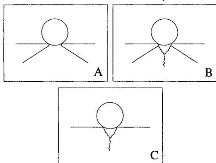
**Figure 1.** Schematic of indentation fracture of graphite with different textures<sup>1</sup>, (spherical tungsten carbide indenter of diameter 6mm was used). A, Poco ZXF, B, EY306, C, IM1-24.
