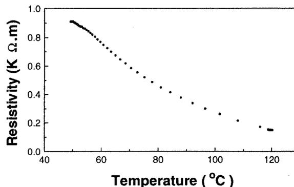
Fig. 2: Electrical resistivity of the sample B as a function of the temperature.
