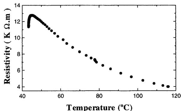
Fig. 1: Electrical resistivity of sample A as a function of the temperature.
