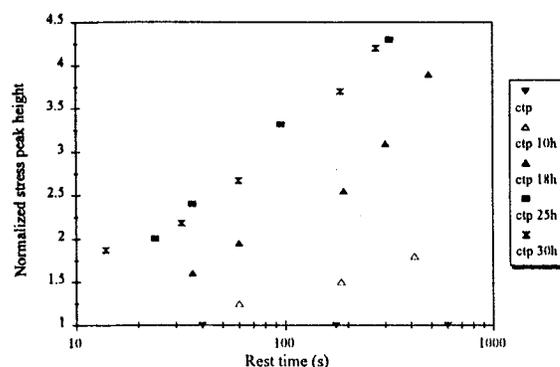
Figure 2. Normalized stress peak height vs. rest time before consecutive start-up of flow for the pitches produced.
