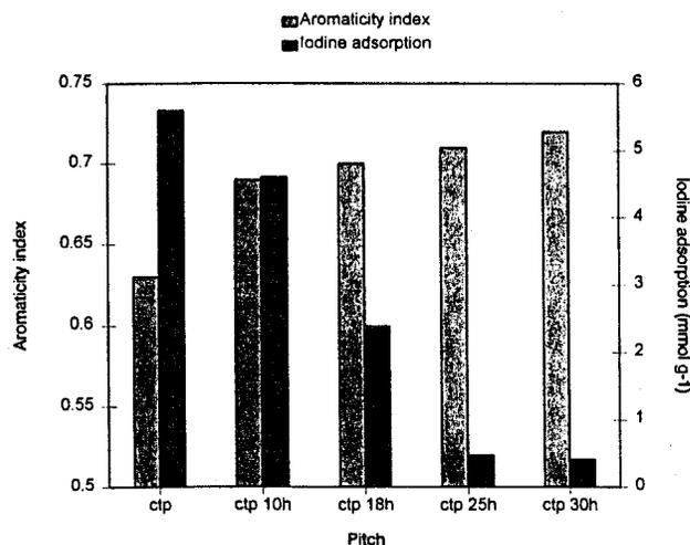
Figure 1. Aromaticity index and Iodine adsorption of pitches
