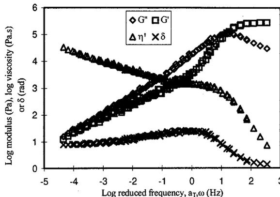
Figure 2. Master curves for Carbores/1 at  $T_g=290^\circ\text{C}$ .
