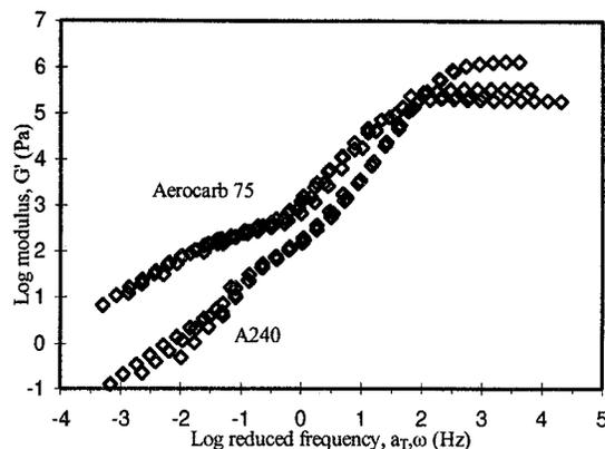
Figure 1.  $G'$  Master curves for A240 and Aerocarb 75.
