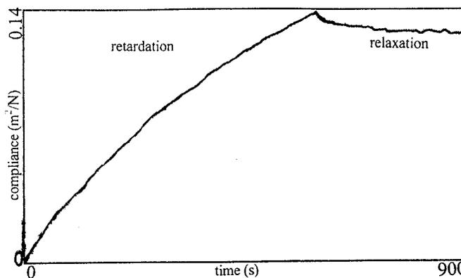
Figure 3. Creep curve of Carbores/1 at  $310^\circ\text{C}$  ( $\sigma=1\text{Pa}$ ).
