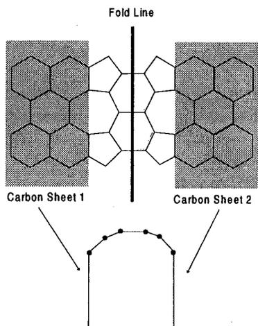
**Figure 3.** An unfolded partial edge at a hole with two carbon sheets.
