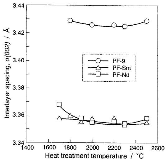
Fig. 3. HTT dependence of  $d(002)$ -spacing of the PF-9, PF-Sm and PF-Nd beads.
