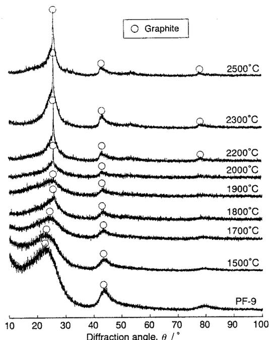
Fig. 1. Effect of HTT on XRD profiles of the PF-9 beads.
