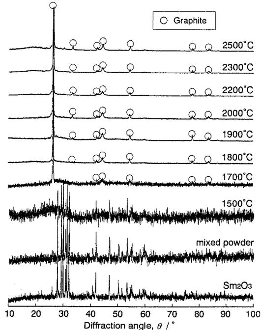
Fig. 2. Effect of HTT on XRD profiles of the PF-Sm beads.
