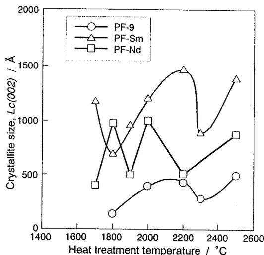
Fig. 4. HTT dependence of  $L_c(002)$  of the PF-9, PF-Sm and PF-Nd beads.
