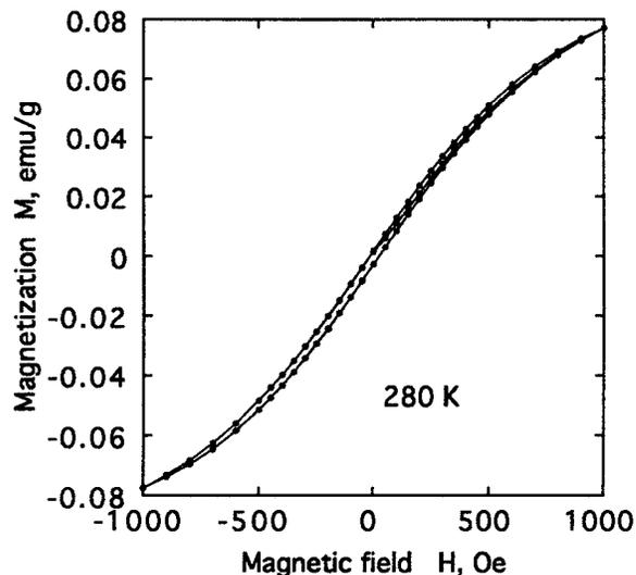
Figure 2. Hysteresis (M versus H) curves in the magnetic field range of  $\pm 1$  kOe for  $C_3N_{3.6}O_{1.1}H_{4.2}$  prepared by the reaction of  $C_3N_3Cl_3$  with  $Li_3N$  under  $N_2$  containing a small amount of  $O_2$ .
