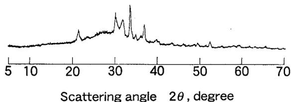
Figure 1. X-ray diffraction pattern of  $C_3N_{3.6}O_{1.1}H_{4.2}$  prepared by the reaction of  $C_3N_3Cl_3$  with  $Li_3N$  under  $N_2$ .
