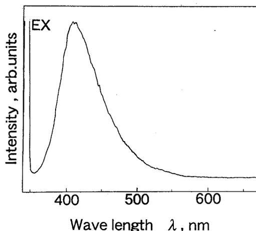
Figure 3. Photoluminescence spectrum at 300K for  $C_3N_{3.6}O_{1.1}H_{4.2}$  prepared by the reaction of  $C_3N_3Cl_3$  with  $Li_3N$ . EX indicates the excitation light of 343nm.
