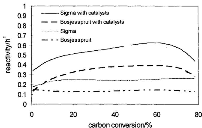
**Figure 1** Carbon conversion profiles for the reaction of Sasol coals with CO<sub>2</sub>.
