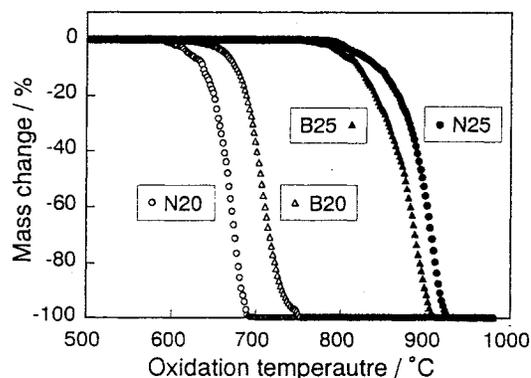
Fig. 2. TGA curves of the films with and without B-doped heat-treated at 2000° and 2500°C.
