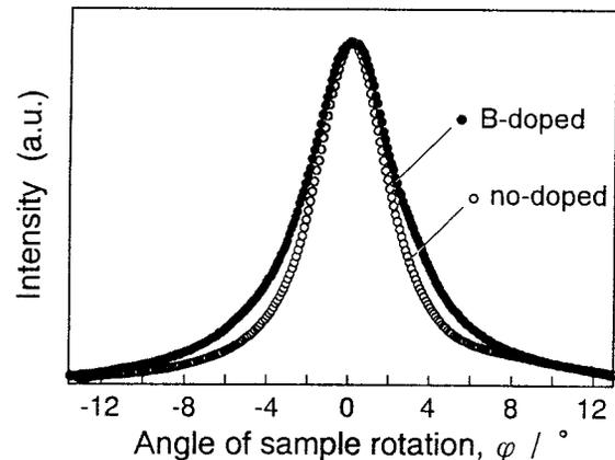
Fig. 4. Orientation of graphite 002 plane of the film heat-treated at 2500°C ; the angle  $\varphi$  is referred to the normal to the specimen surface at the diffraction angle giving the 002 intensity maximum.
