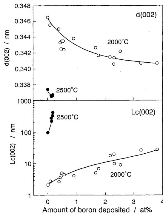
Fig. 1. Change of  $d(002)$  and  $L_c(002)$  for the films heat-treated at 2000° and 2500°C with amount of boron deposited.
