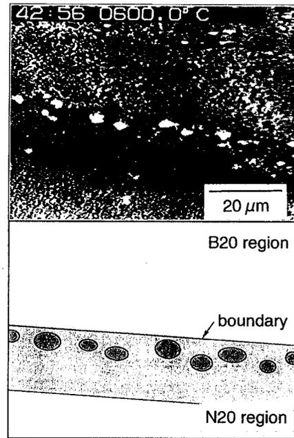
Fig. 3. LM in-situ observation and illustration of morphological changes in the process of oxidation at 600°C for the film heat-treated at 2000°C.
