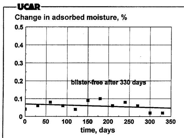
Figure 3. Surface stability study with 1000°C hydrogenated flexible graphite.
