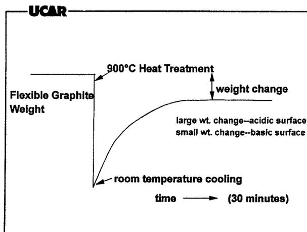
Figure 1. Flexible graphite surface test.
