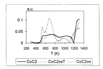
**Figure 1.** Temperature-programmed reduction profiles for fresh Co/AC2, Co/AC2 $_{ox}$  and Co/AC2 $_{ox}$ T catalysts.
