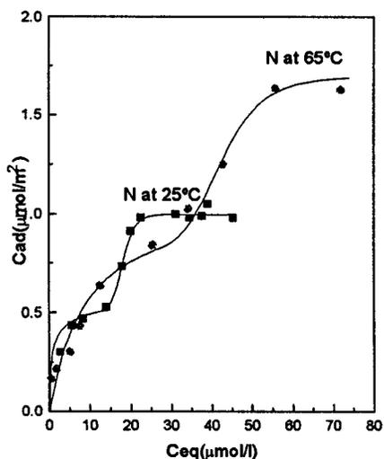
Figure 1. Nonylphenol adsorption isotherms on carbon N
