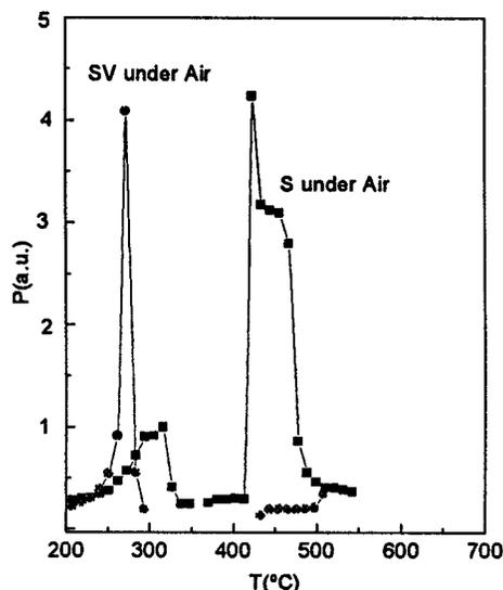
Figure 3. Desorption of nonylphenol during thermal regeneration of carbon S with and without V
