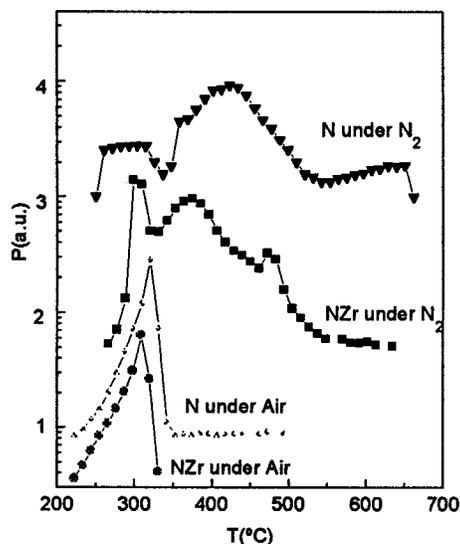
Figure 2. Desorption of nonylphenol during thermal regeneration of carbon N with and without
