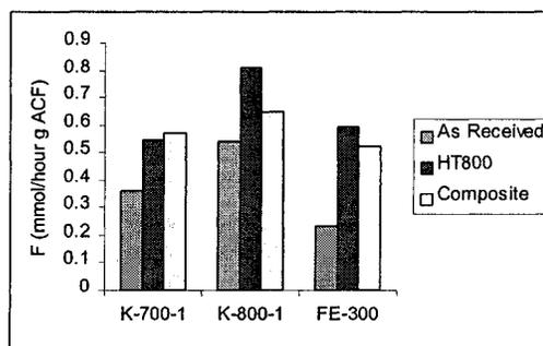
Figure 3. Catalytic activity for as-received ACF, heat-treated 800°C, and ACF composites.
