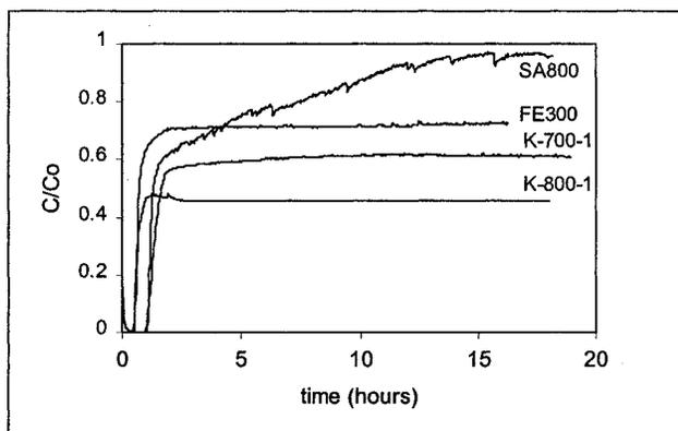
Figure 2. SO<sub>2</sub> breakthrough plots for as received ACF.
