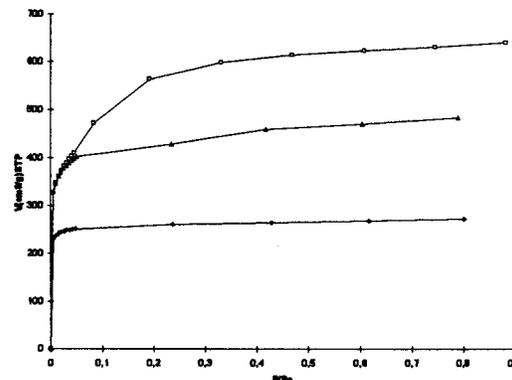
Figure 1, adsorption isotherms on microporous carbons. □ SeS, Saarkohle swollen coal burn-off 70% ; Δ CeS, Cerrejón swollen coal burn-off 30%, ♦ Ce, Cerrejón coal burn-off 70%
