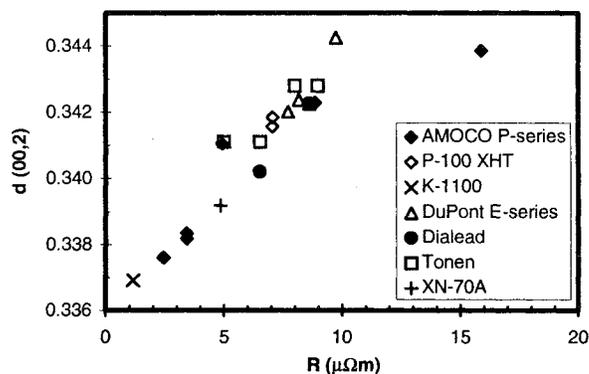
Figure 2. Spacing between graphene planes,  $d_{(00,2)}$ , and electrical resistivity,  $R$ , in carbon fibers.
