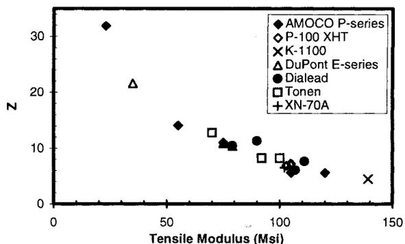
Figure 3. Fiber c-axis orientation,  $Z$ , and carbon fiber tensile modulus.
