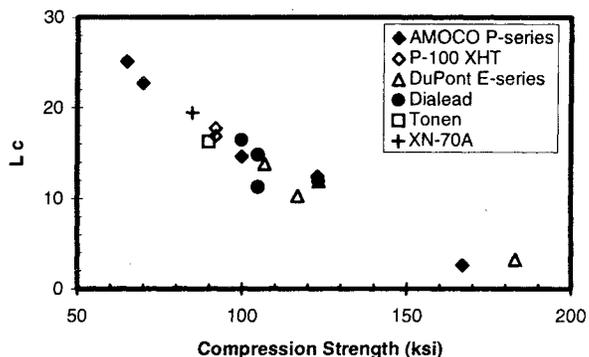
Figure 4. C-axis crystallite size,  $L_c$ , and carbon fiber compression strengths.
