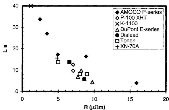
Figure 1. In-plane graphitic crystal size parallel to the fiber axis,  $L_a$ , and electrical resistivity,  $R$ , in carbon fibers.
