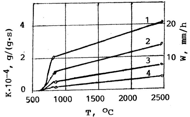
FIGURE 1: Dependence of the mass loss rate (1, 2) and sample diameter reduction (3, 4) of unimpregnated (1, 3) and impregnated (2, 4) graphite on the temperature of oxidation
