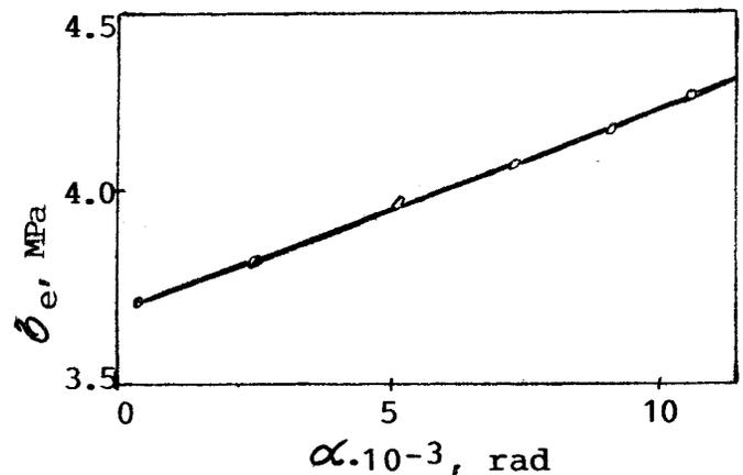
FIGURE 2: The influence of the degree of oxidation of 610 mm diameter electrode on the value of maximum equivalent stresses
