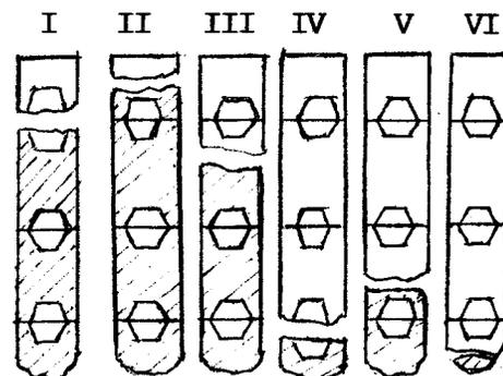
FIGURE 3: Typical breakages of electrodes during operation
