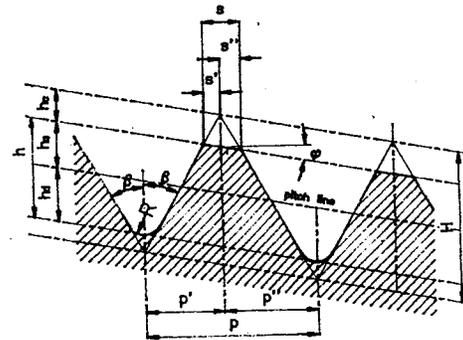
Fig. 1. --- Illustration of taper thread profile.
