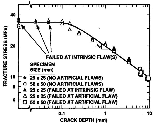
Figure 2. Fracture stress versus flaw depth for IG-11 graphite
