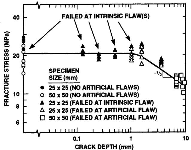
Figure 3. Fracture stress versus flaw depth for H-451 graphite
