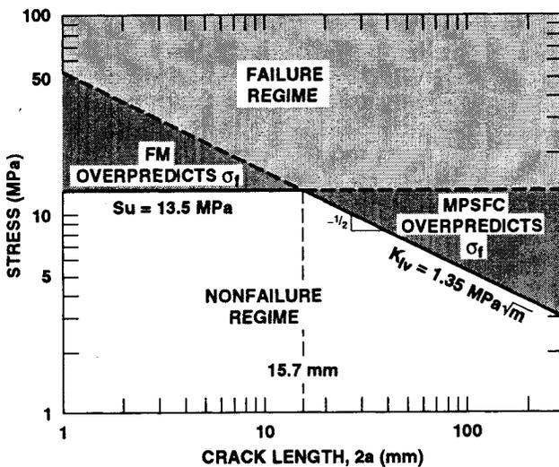
Figure 1. Fracture stress versus crack length for H-451 graphite
