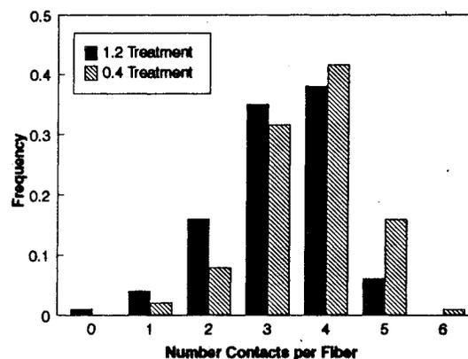
Fig. 2. Fiber contact density distributions for two T40R/phenolic laminates of different surface treatments.
