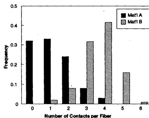
Fig. 1. Histograms for fiber-contact densities of two composites. A: T300/phenolic, with .58 fiber volume fraction; B: T40R/phenolic, with .79 fiber volume.
