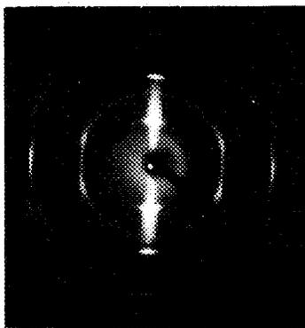
Figure 2 -- Precession XRD of pristine P-100 fiber.
