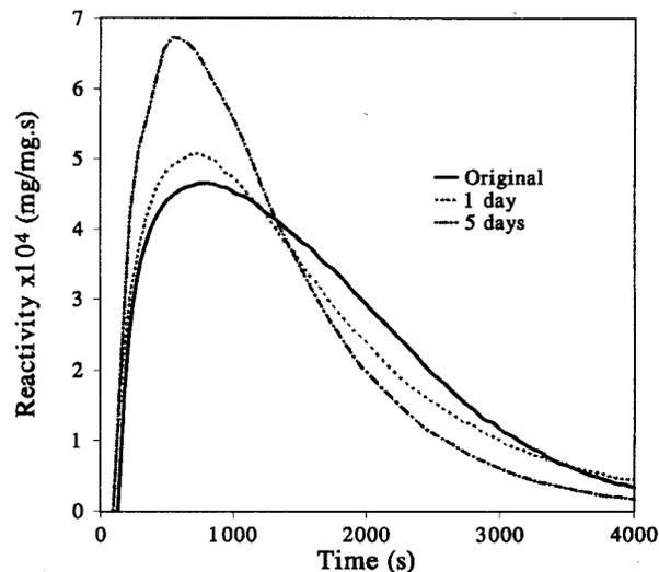
Figure 2. Evolution of the instantaneous reactivity for fresh and oxidized Tu coal.
