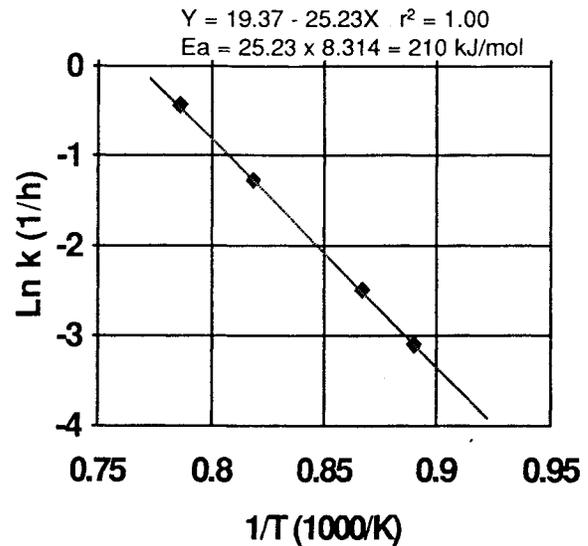
Fig. 2 Arrhenius plot of CO<sub>2</sub> activation rate of carbon fibers against activation temperature.
