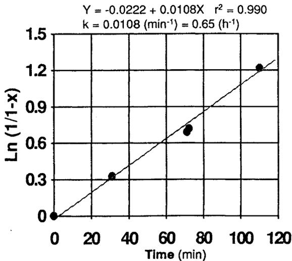
Fig. 1 Plot of a kinetic parameters against reaction time for CO<sub>2</sub> activation of fibers carbonized at 850°C.
