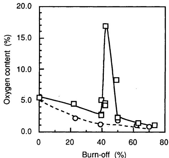
Fig. 3. Change in oxygen content of fiber as a function of burn-off: (□), in CO<sub>2</sub>; (○), in steam.
