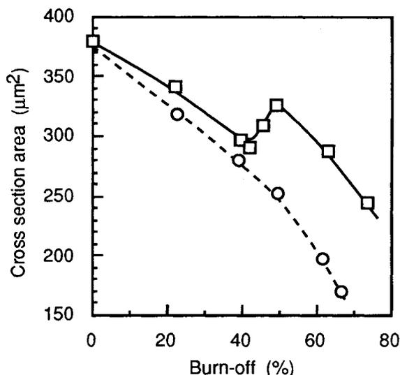
Fig. 2. Change in cross section area of fiber as a function of burn-off: (□), in CO<sub>2</sub>; (○), in steam.
