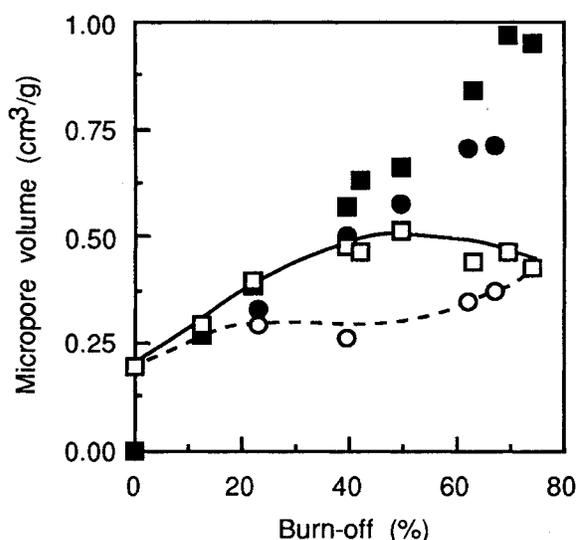
Fig.1. Micropore volume vs burn-off: ( $\square$ ), V<sub>nar</sub> and ( $\blacksquare$ ), V for CO<sub>2</sub> activation; (O), V<sub>nar</sub> and ( $\bullet$ ), V for steam activation.
