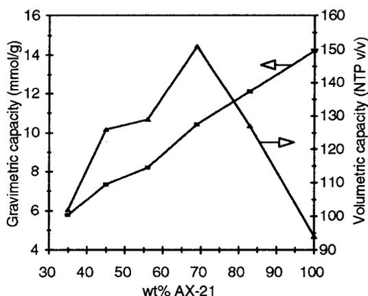
Figure 1 Volumetric and gravimetric capacities of methane in AX-21/resin monoliths
