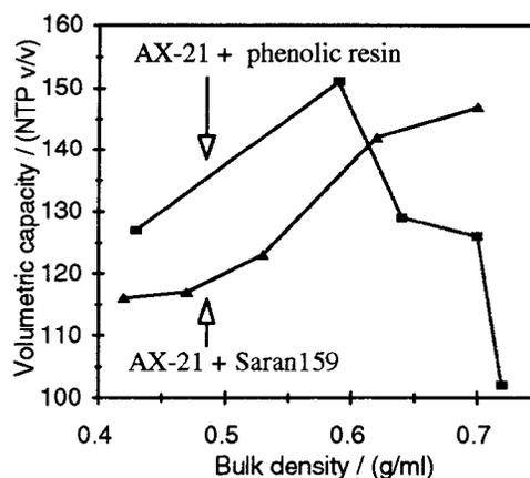
Figure 2 Comparison of volumetric capacities of AX-21 carbon monoliths
