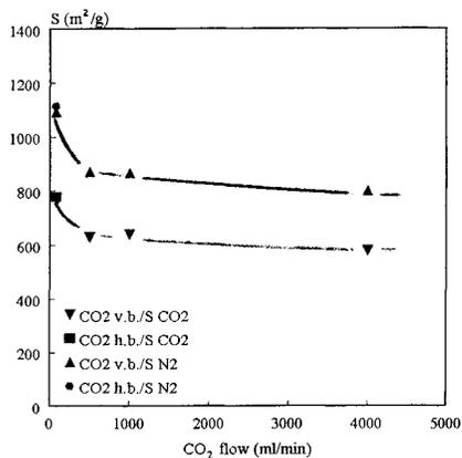
Figure 2. Variation of the apparent surface area as function of CO<sub>2</sub> flows. (▲ N<sub>2</sub> BET, ▼ CO<sub>2</sub> DR)
