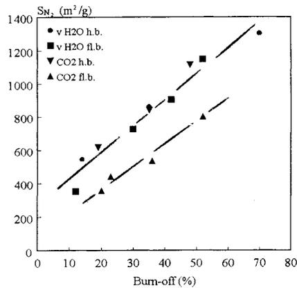
Figure 1. Variation of the apparent surface area versus burn-off.
