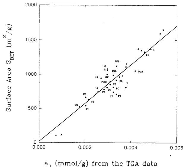
**Figure 2** - Linear relationship between the BET specific surface area evaluated from argon adsorption data and the TGA weight-loss II (see Figure 1) obtained for n-butanol. Symbols at experimental points denote various active carbons.
