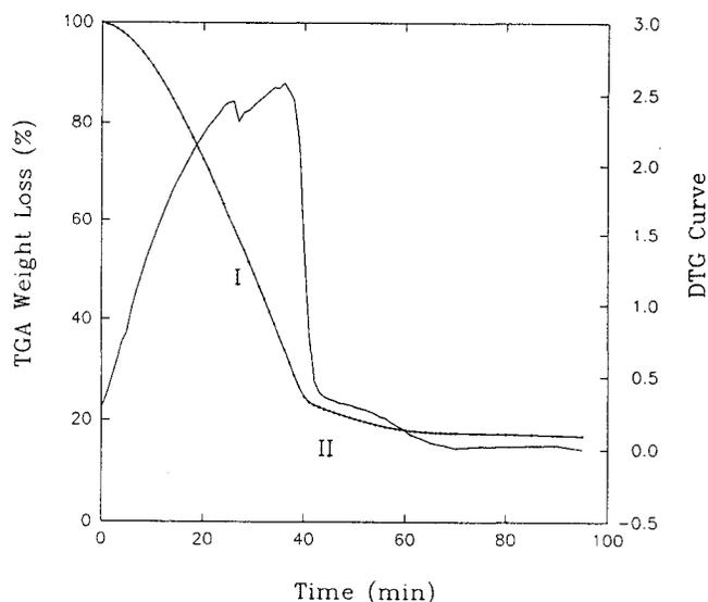
**Figure 1** - The TGA weight-loss curve and its derivative (DTG) for thermodesorption of n-butanol from an active carbon. The points I and II refer respectively to the total adsorption capacity (total porosity) and the amount adsorbed in the pore walls.
