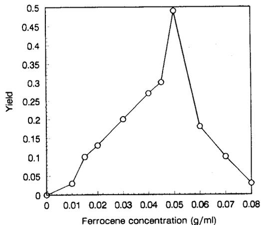
Fig.2 A plot of VGCFs yield against the Ferrocene concentration
