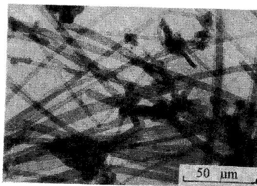
Fig.5 The micrograph of VGCFs
