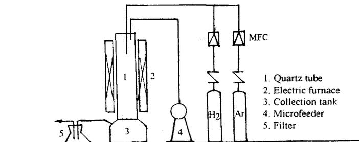
Fig.1 Schematic diagram of the apparatus for preparing VGCFs
