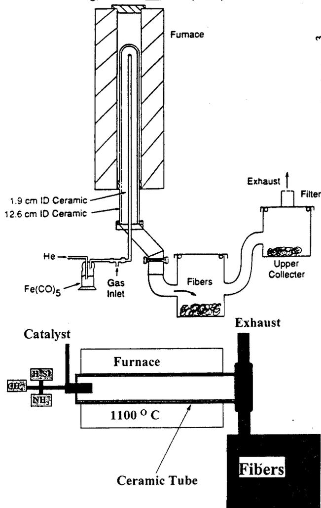
Figure 1. The top panel shows the vertical reactor with a 1.9 cm ID injector inserted 89 cm into the 12.6 cm ID tube of heated length 95 cm. The bottom panel shows the horizontal apparatus whose injector is a 2 cm ID tube inserted 30 cm into a 10 cm ID tube of heated length 183 cm. All tubes are of mullite.
