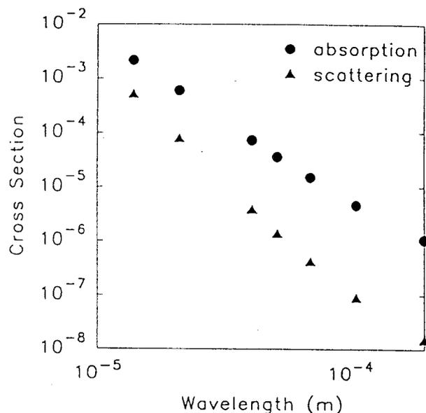
Fig. 2: Cross sections of VGCF vs. wavelength.
