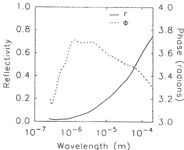
Fig. 1: Reflectance and phase of VGCF vs. wavelength.
