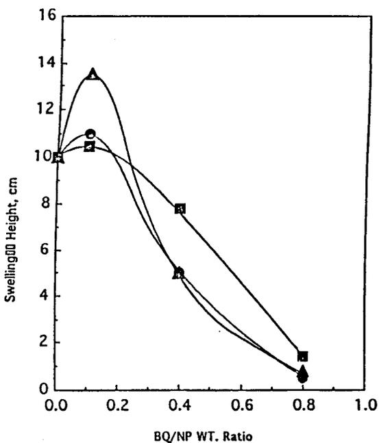
Fig. 1. Swelling height dependence on the BQ/NP weight ratio : heat treated at 300°C; carbonized at 600°C.
