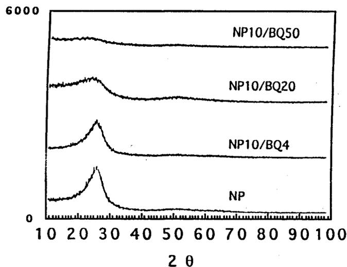
Fig. 2. X-ray diffractions of the carbonized samples at various BQ weight ratio ; carbonized at 600 °C.
