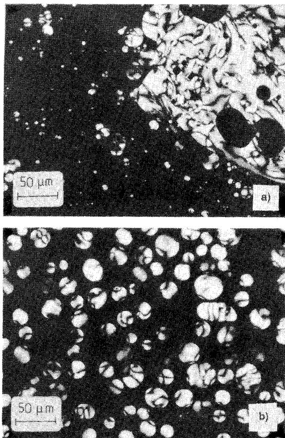
**Fig. 1.** Optical micrographs of mesophase pitches produced at 440°C and 5h residue time without (a) and with iron benzoate (b).
