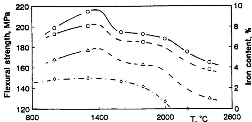
**Fig. 2.** Flexural strength and iron content in dependence of heat treatment temperature; ○, 18%; □, 22%; △, 15% penetration; ◇, iron content.
