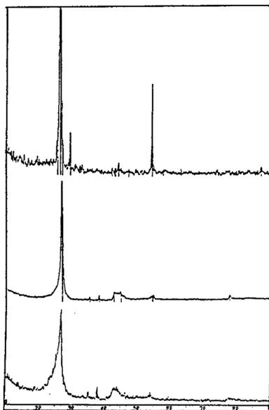
Figure 2, X-ray diffractions of B/C materials prepared at 1800 °C (a), 2100 °C (b) and 2300 °C (c).
