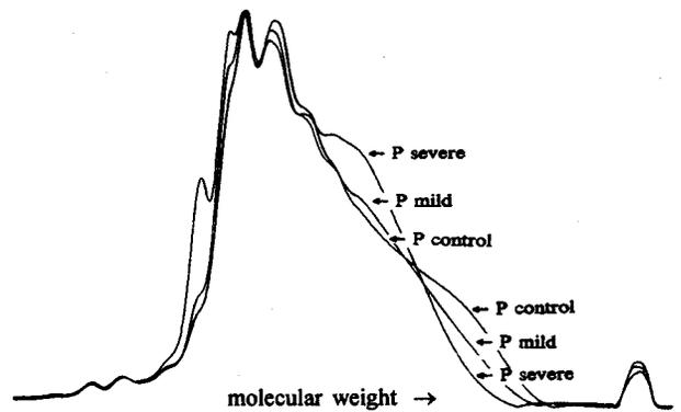
Figure 3: Comparison of GPC curves from pitches made from a single coal-tar source with different levels of thermal treatment.
