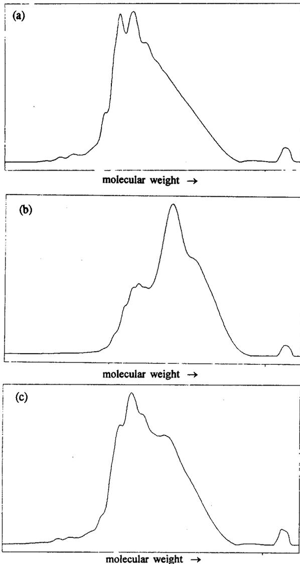
Figure 1: GPC chromatograms of (a) a typical coal-tar pitch, (b) a typical petroleum pitch, and (c) a pitch made from both coal-tar and petroleum precursors.
