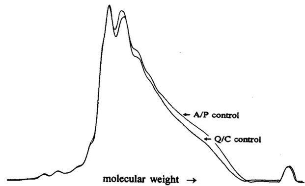
Figure 2: Comparison of GPC curves from pitches made with different coal-tar precursors.
